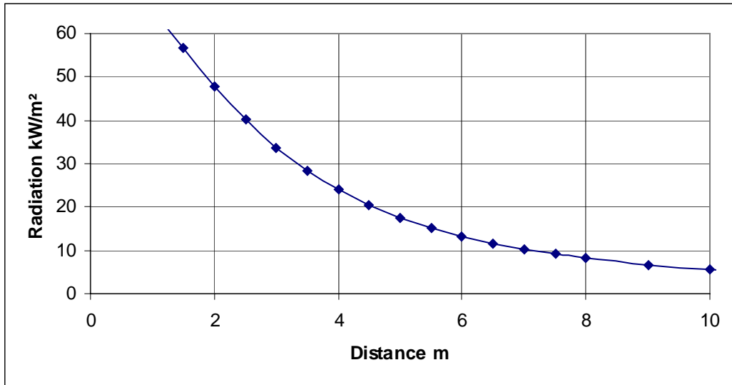
Figure 6. Heat radiation v. distance when the demountable platform is burning.
